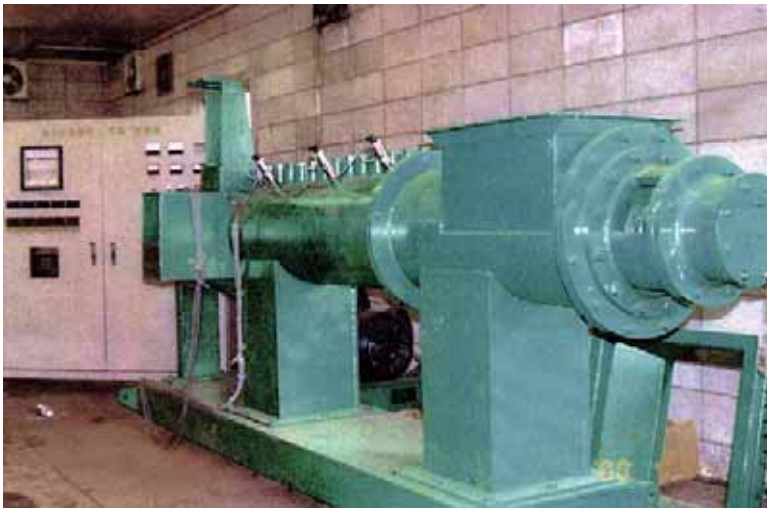
Photograph 1 Normal temperature, normal pressure and high shearing stress type Kneader for testing (shearing stress is 0.4-1.0 M Pascal, capacity of 200 liters)
