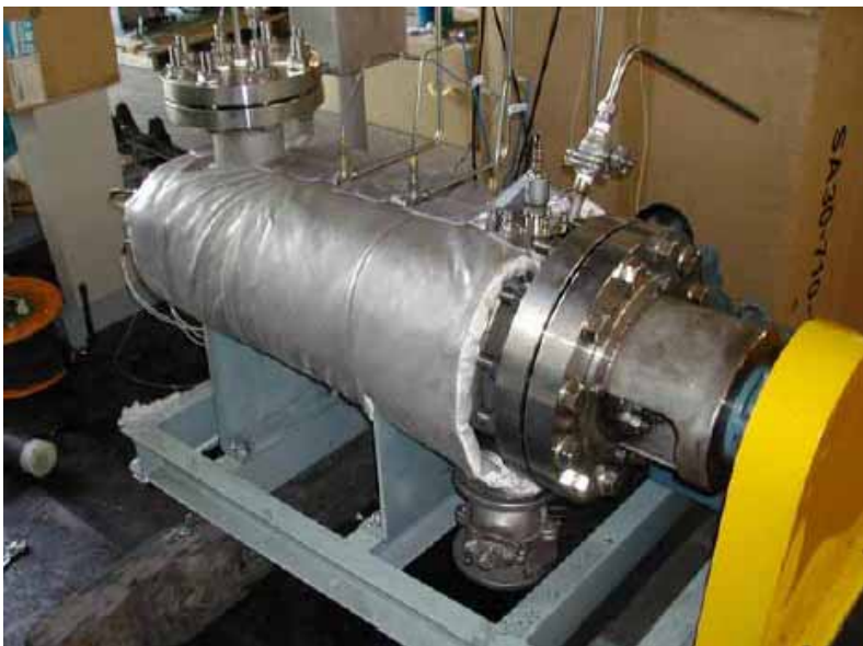
Photograph 2 High temperature, high pressure, and high shearing stress type Kneader for testing (shearing stress is 0.4-1.0 M Pascal, capacity of 30 liters) (The same device as newspaper announcement)
